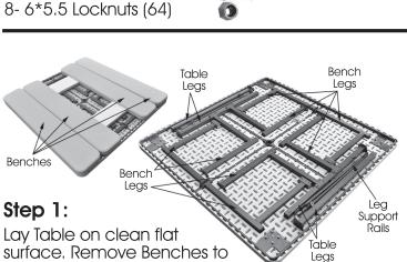
expose all the assembly parts and hardware bag. Unload these parts and begin assembly.
